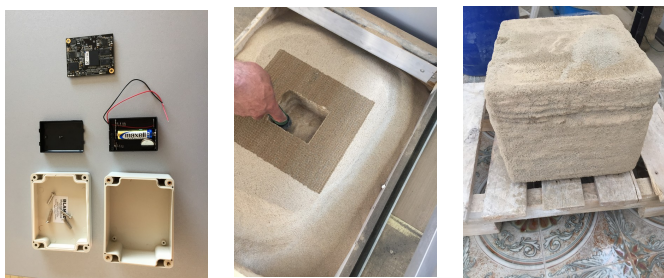
Fig. 2. Insertion of a LoRaWAN End Device within an artifact
