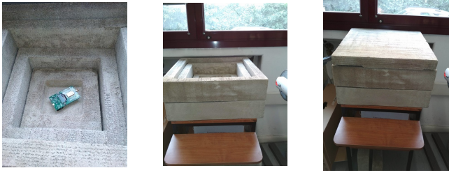
Fig. 4. LoRa End Device inserted in the modular cube for communication tests
