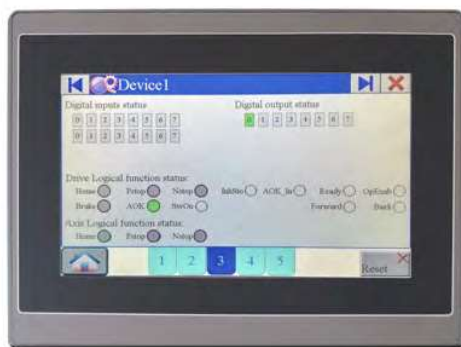
PT2 HMI here with one of available CMZ libraries configured for a flowpack
