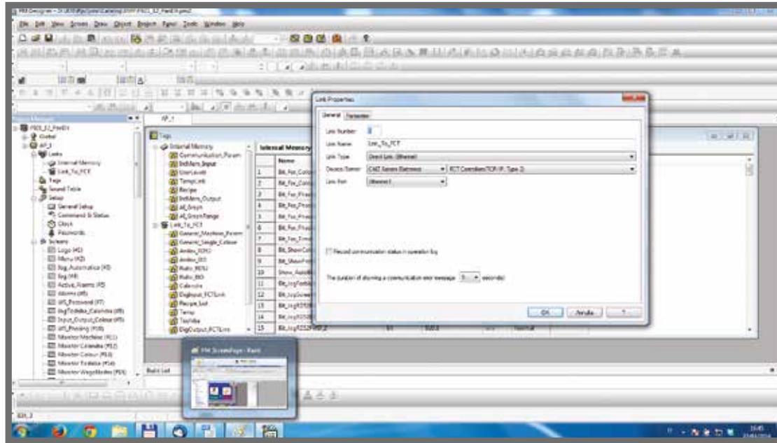
The PM Designer is a simple and intuitive development environment that, without the need of any other software instrument, allows to realize the GUI (Graphical User Interface) and to program the functionalities of the CMZ operator panels. This single environment allows the programming and the download of the applications in all the HMI models that the CMZ provides of PT2 series.
