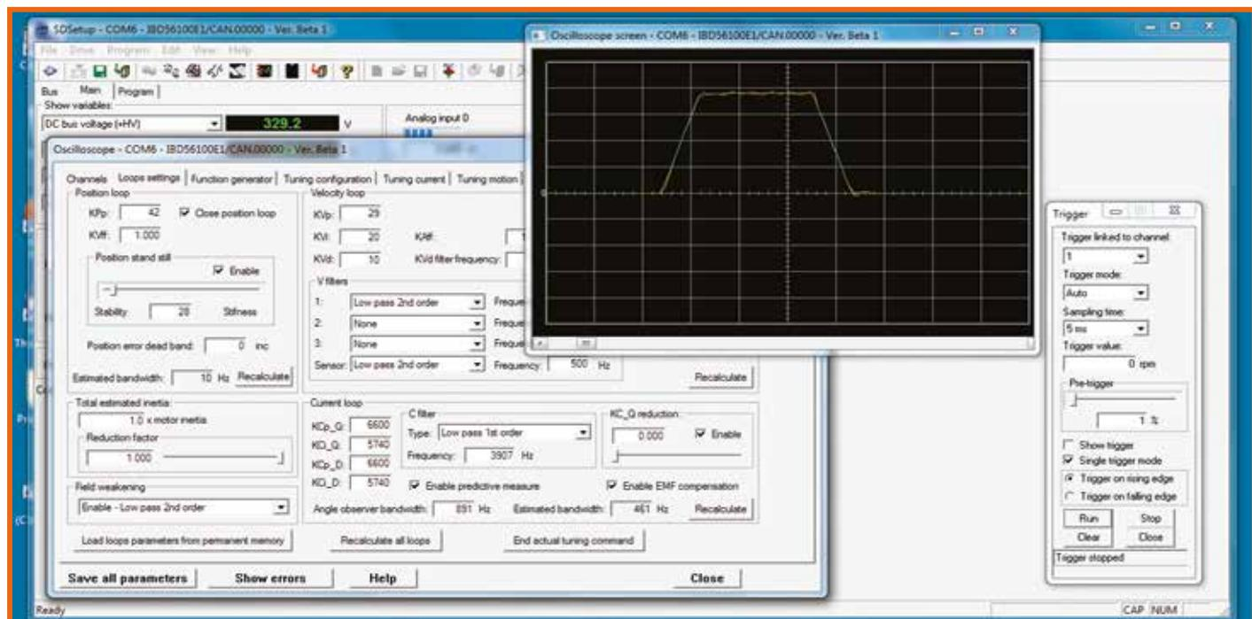
**SD setup** is the development environment for the configuration, parameterization, tuning and programming of the drives ISD/SVM and IBD/NBD using the RS232 serial connection or a centralized connection through a fieldbus when the master controller is a controller of the FCT family.
