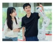
ABB Robotics has launched a six-axis robot aimed at the education sector. The 21kg IRB 1090 robot offers a reach of 580mm and a payload of 3.5kg. It is 20% lighter than its predecessor and has a 10%
